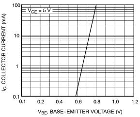
Figure 2. Transfer Characteristics
