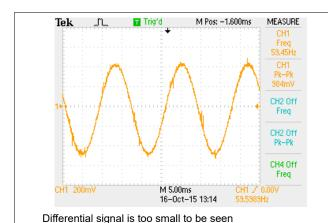
Figure 8-4. Common-mode Signal at INA126 Input
