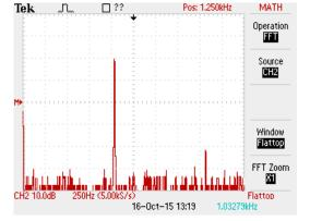
Figure 8-7. FFT of the INA126 Output Shows that the 60-Hz Common-mode Signal is Rejected
