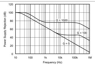
Figure 6-3. Positive Power Supply Rejection vs Frequency
