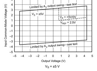
Figure 6-5. Input Common-Mode Voltage Range vs Output Voltage
