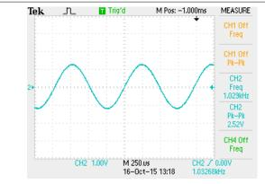
Figure 8-6. Recovered Differential Signal at the Output of the INA126 With a Gain of 250
