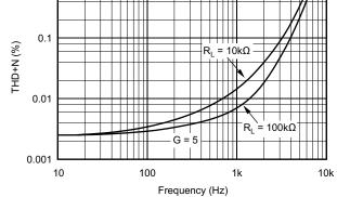
Figure 6-12. Total Harmonic Distortion + Noise vs Frequency
