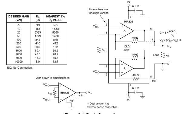
Figure 8-1. Basic Connections
