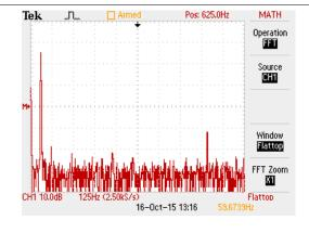
Figure 8-5. FFT of Signal in Previous Figure Shows Both the 60-Hz Common-mode Along With 5-kHz Differential Signal
