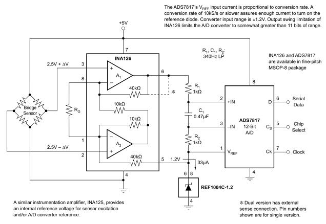
Figure 9-1. Bridge Signal Acquisition, Single 5-V Supply
