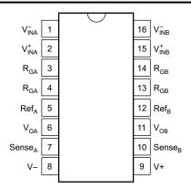
Figure 5-2. INA2126: N (16-Pin PDIP), D (16-Pin SOIC), and DBQ (16-Pin SSOP) Packages, Top View
